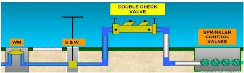
The service connection double check valve should prevent contamination of the main pipes, from the residential service, but each property owner is required to have a few additional measures to prevent cross-connections that would possibly cause a contamination within their own system.
